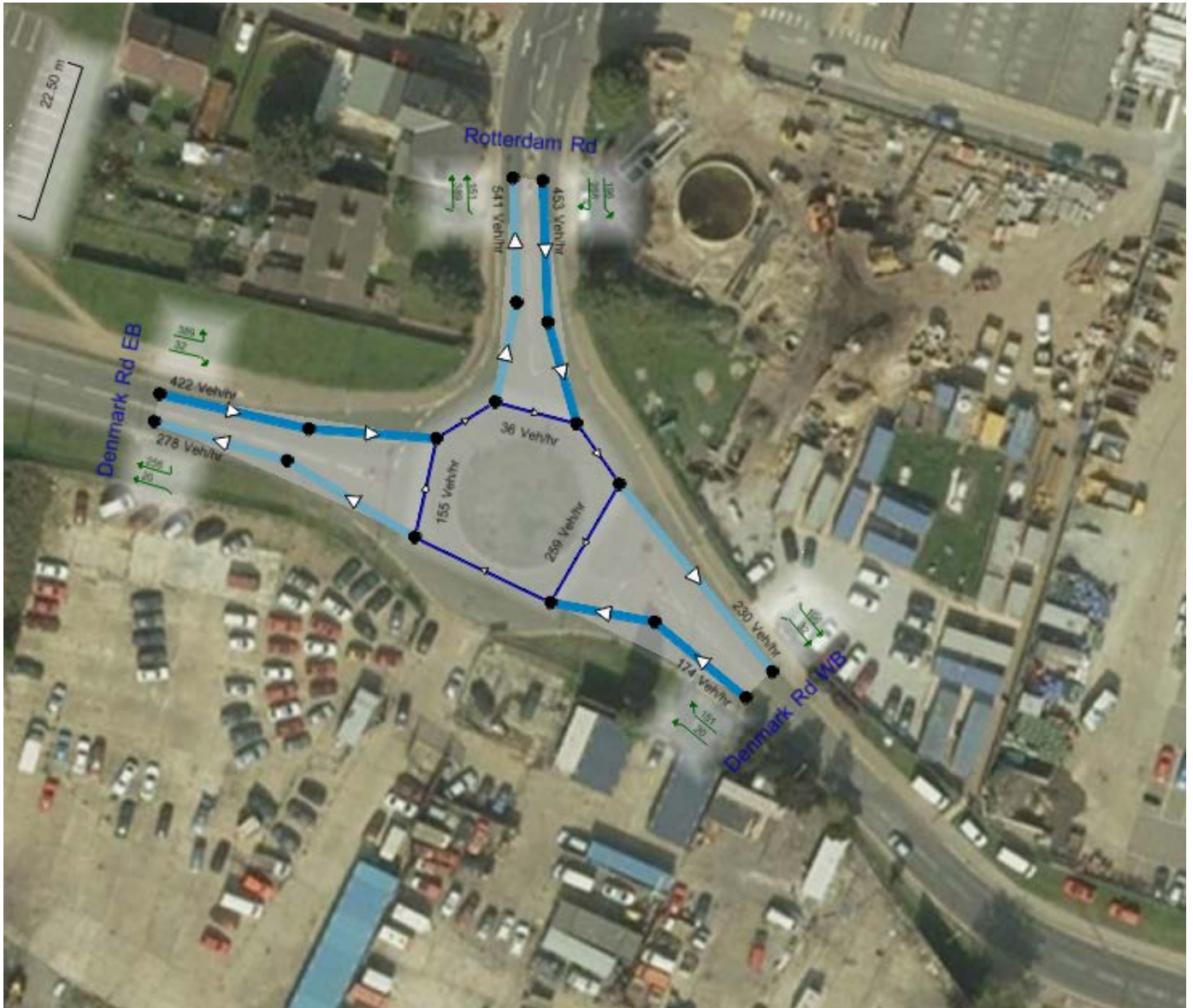
The junction diagram reflects the last run of ARCADY.
